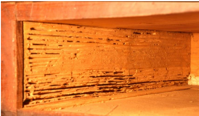
Manastero S. Nicolò all'Arena (CT) Italy. Library and Sacristy furnitures. Termites damage
