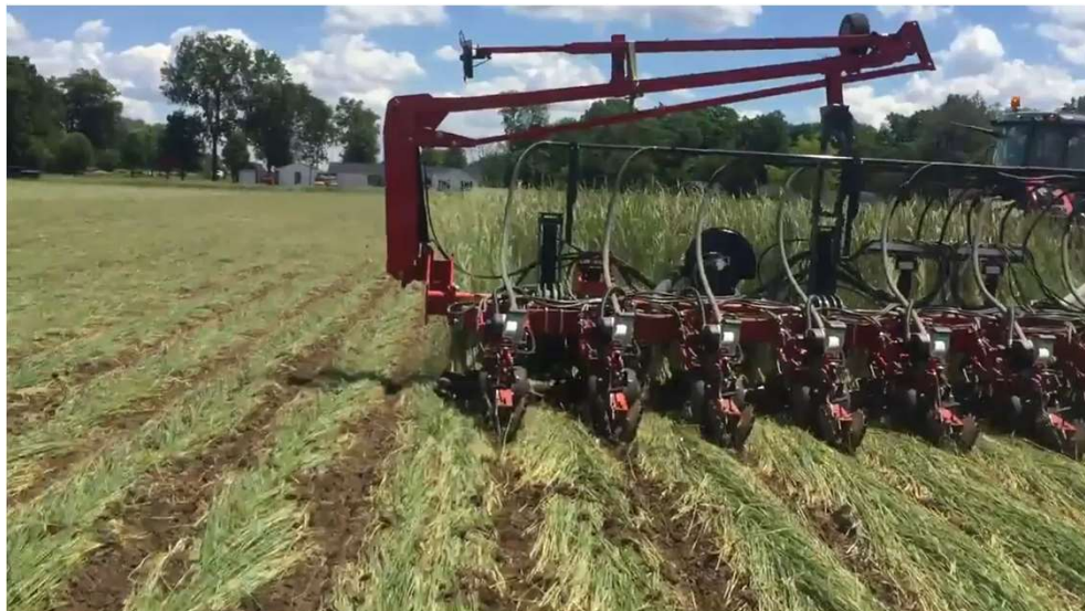
ZRX Roller Crimper in Cereal Rye with 24 row AGCO planter
